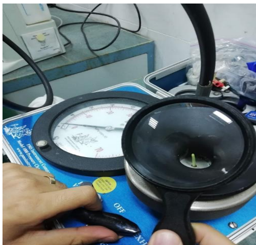
Figure 3. Measurement of leaf water potential by using pressure
