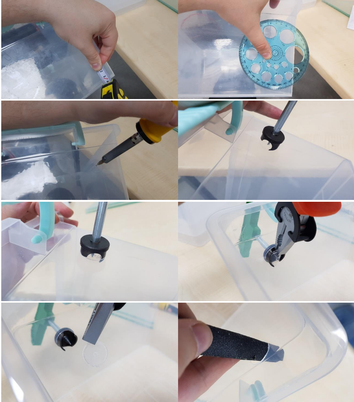
Figure 1. Processes of the drilling water inlets and outlets by using different equipment.
